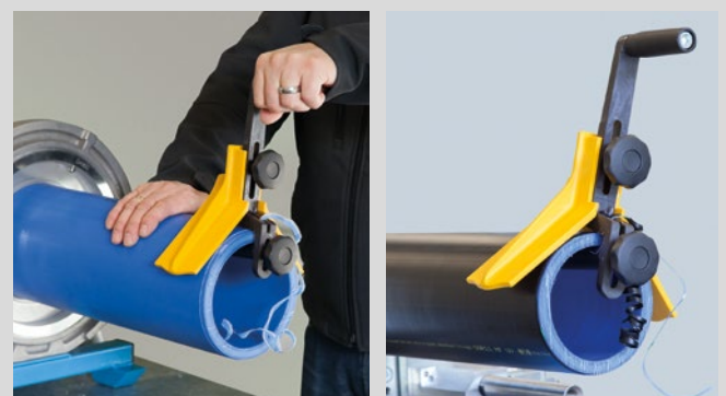
Chamfering of the front side in case of the OT and UV pipe
