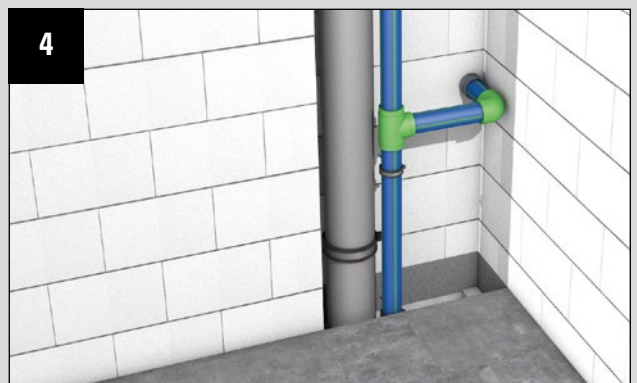
Installation of a spring leg
